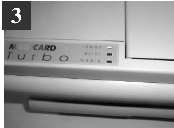
3 Switch ON. The indicators should all flash and the motors run briefly. Finally, the READY LED will remain ON.
